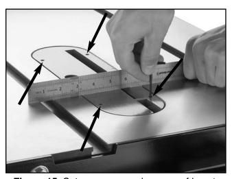
Figure 15. Setscrews on each corner of insert.
